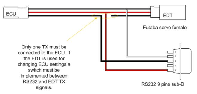
If an EDT is used which can alter the settings of the ECU the TX of the EDT can't be connected directly to the ECU. A collision will take place between the TX signals of the RS232 connection and from the EDT. If both connections are preferred a switch must be implemented for switching between TX signal of the RS232 connection and the TX signal of the EDT.
